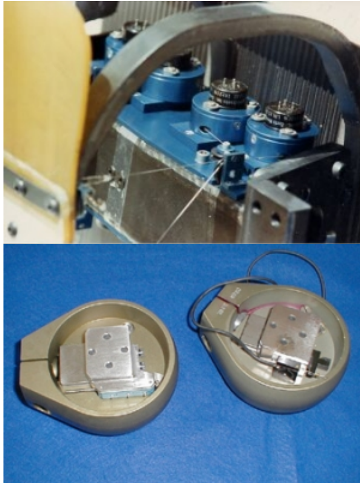
Figure 11 - Crash test dummies get smart with Firstmark Controls position transducers
